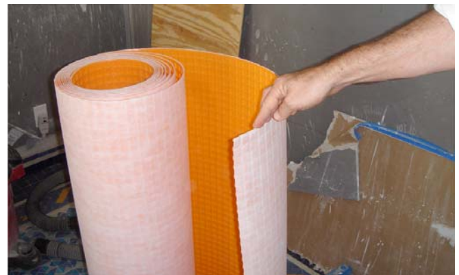
Photograph 10: Dimpled Plastic Sheet Membrane
