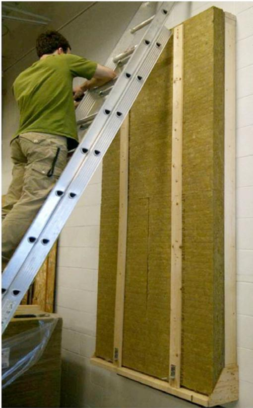
**Photograph 3: Detailed Test (left)**—The simple tests get you enough information to do more detailed tests. The deflection testing shown here is at our Skunk Works.
