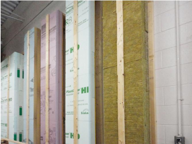
**Photograph 1: Build Stuff and Break It**—The only way to know is to test it to failure and then you know. How do you figure out how to attach cladding through various types of rigid insulation? You build a whole bunch of assemblies and see. There is no other way.
